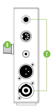
Note that you're able to check cable status between different connectors. Some of the more common examples are: XLR, RCA or I/8" (3.5mm) to I/4" (6.35mm).
